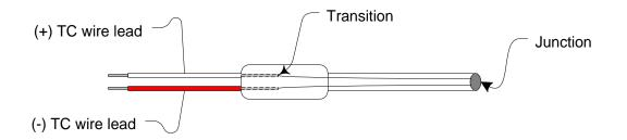
When the ground between the tool-mold connector-controller is missing or becomes worn (forms a slight resistance), the next best ground path is through the thermocouple wire. This then exposes two major weaknesses present today in all cases.
